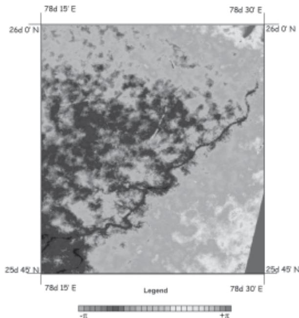
**Fig. 3.** Interferogram of Sind region generated from ERS-1/2 SAR SLC tandem data.
