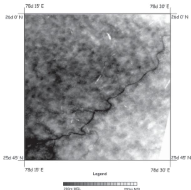
**Fig. 4.** Digital Elevation Model of Sind river basin generated by SAR interferometry using ERS-1/2 tandem data
