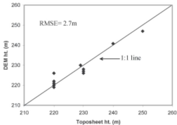
**Fig. 6.** Comparison of altitudes of check points from toposheet survey and from interferometric DEM
