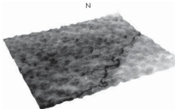
**Fig. 5.** Vertically exaggerated perspective view of the DEM generated by SAR Interferometry
