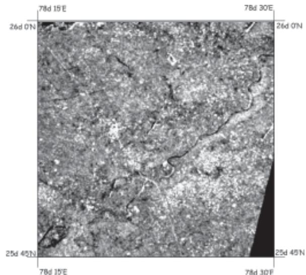
**Fig. 1.** Intensity image of the Sind region derived from ERS-1 SAR SLC data (Master image)
