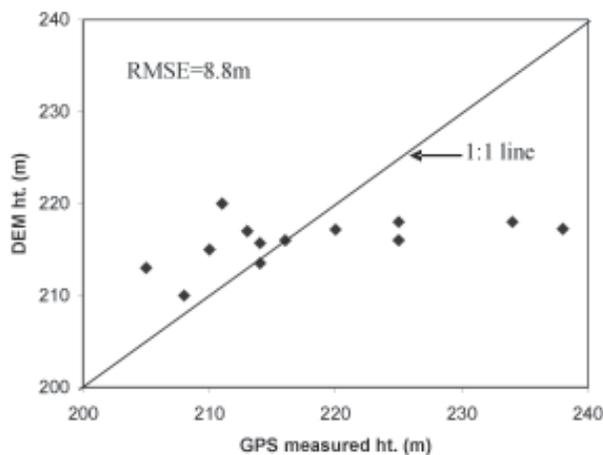
**Fig. 7.** Comparison of altitudes of check points by GPS survey and from interferometric DEM
