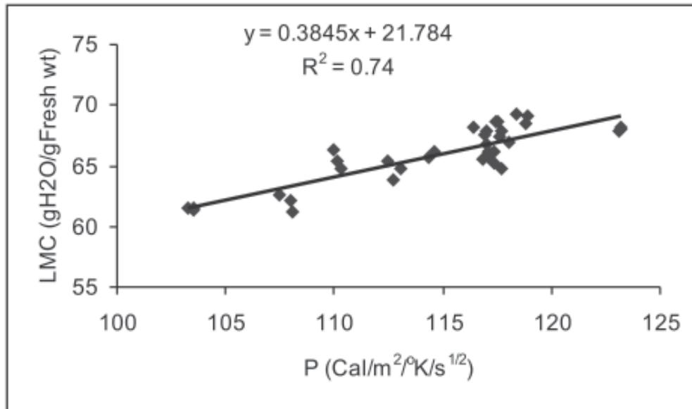
Fig. 1. Leaf moisture content calibration curve against thermal inertia, P
