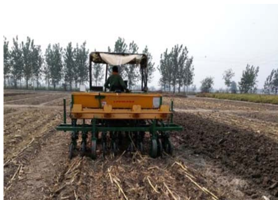
Fig. 9. Inclined plate planter with double disc furrow openers sowing wheat MW system on PRBs (left) and earthing up/weeding in PRBs in wheat (right). (Source: BISA, Ludhiana)
