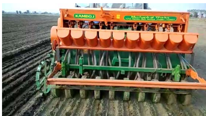
Fig. 6. Happy Seeder with inclined plate attachment for sowing rice, maize and other crops
