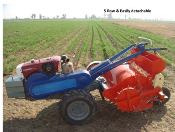
Fig. 11. Turbo Happy Seeder coupled to a 2WT (left) and low powered 4WT (18 hp) (Right) (H.S. Sidhu, BISA Ludhiana).
