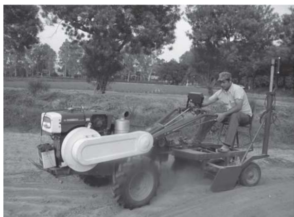
Fig. 12. 2WT driven laser-assisted precision land leveller for small-holder farmers
