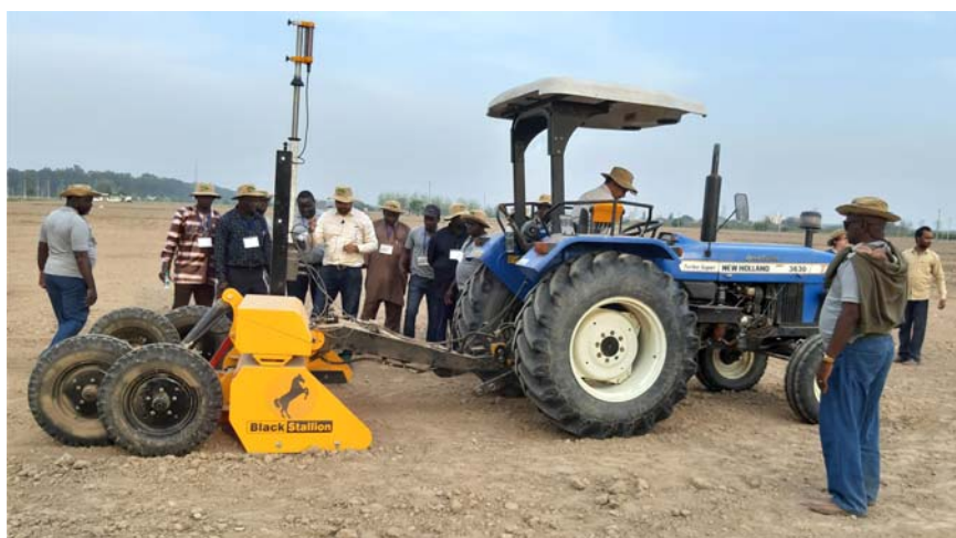
Fig. 1. Field Demonstration of laser land leveller to trainees from West Africa at BISA, Ludhiana
