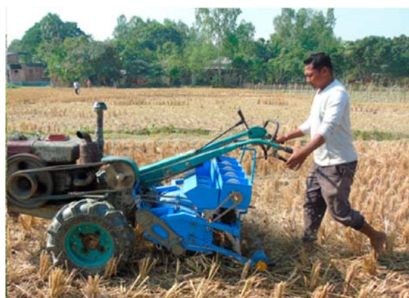
Fig. 13. Versatile multi-crop planter (VMP) attached to a two-wheel tractor (Bell et al. , 2019)
