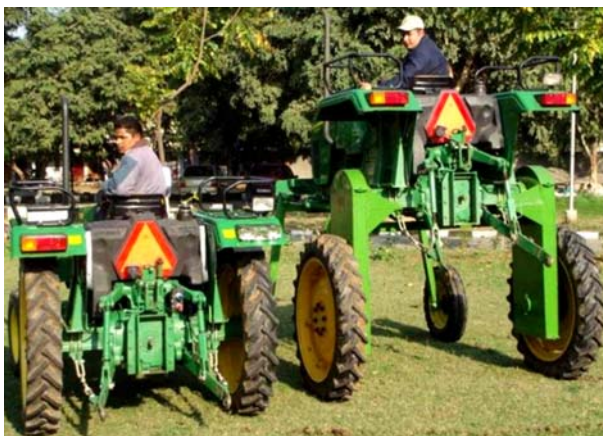
Fig. 8. Normal tractor and mounted on high clearance platform (left) and 15-row relay seeder with ZTDD openers relay seeding wheat into standing cotton (right) (Source: Manpreet-Singh et al. , 2016)
