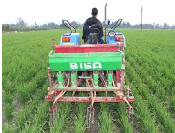
Fig. 10. Band placement of fertilizer nitrogen in wheat using double disc planter nitrogen (Source: R.K. Jat, BISA, Pusa, Bihar, India)
