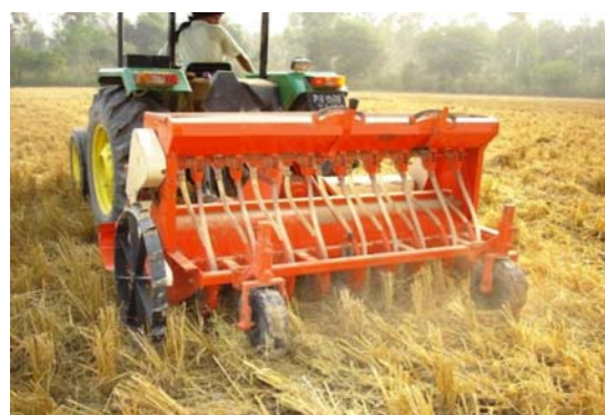
Fig. 2. Turbo Happy Seeder sowing wheat into rice residue
