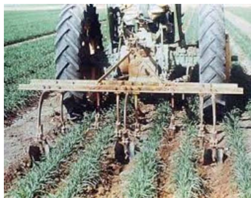
Fig. 9. Inclined plate planter with double disc furrow openers sowing wheat MW system on PRBs (left) and earthing up/weeding in PRBs in wheat (right). (Source: BISA, Ludhiana)
