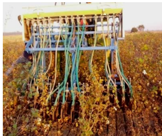
Fig. 8. Normal tractor and mounted on high clearance platform (left) and 15-row relay seeder with ZTDD openers relay seeding wheat into standing cotton (right) (Source: Manpreet-Singh et al. , 2016)
