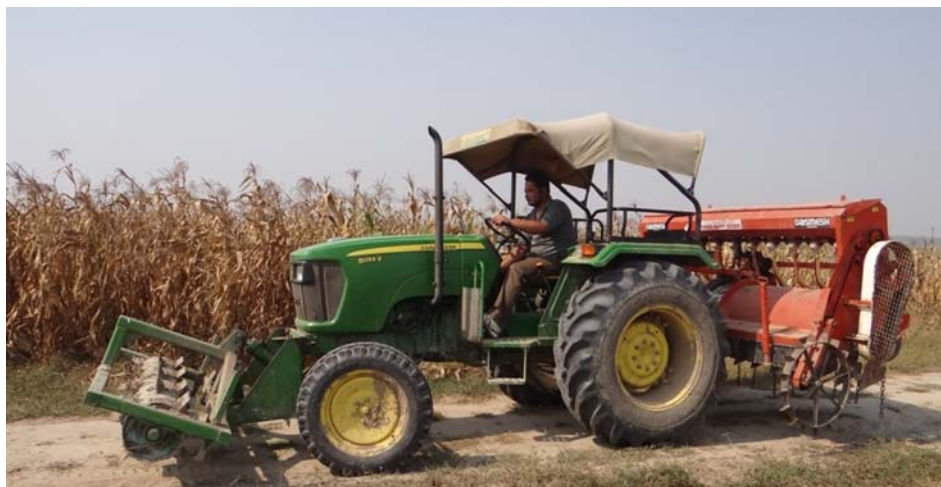
Fig. 7. Knife roller with Turbo Happy Seeder for sowing wheat into maize residues
