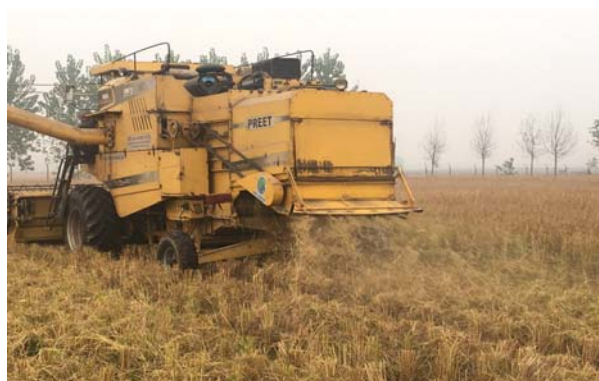
Fig. 3. Combine harvester with Super SMS attachment while harvesting rice
