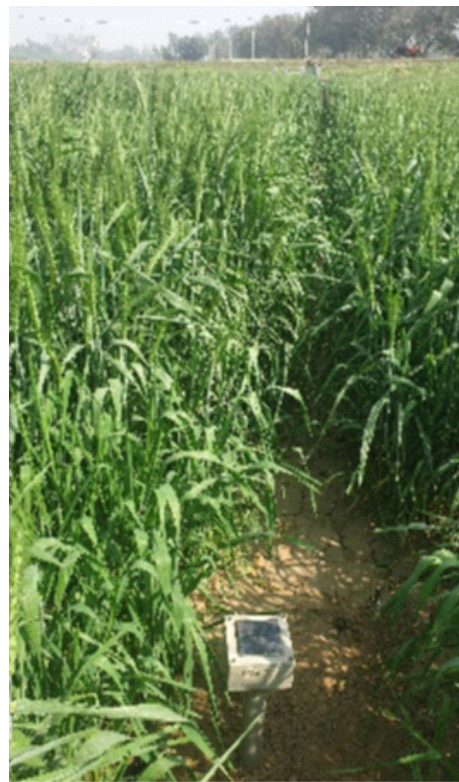
Fig. 2. Solar-operated automatic-check gate and soil moisture sensor installed in the field
