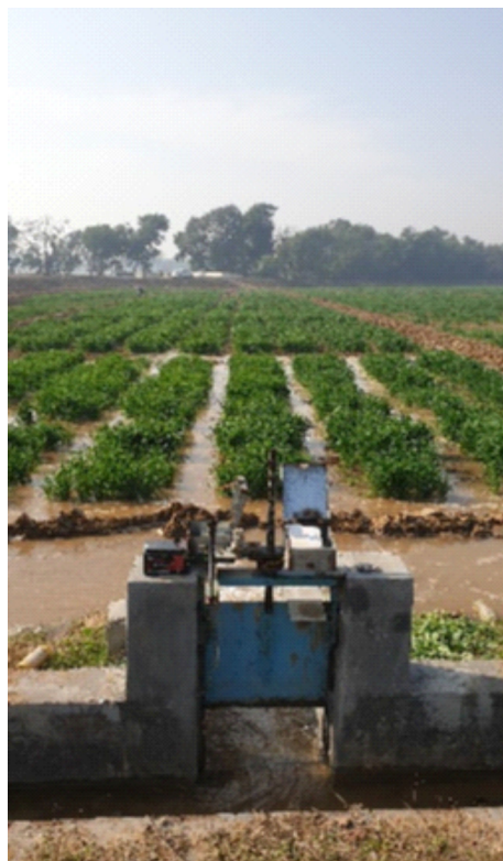
Fig. 2. Solar-operated automatic-check gate and soil moisture sensor installed in the field
