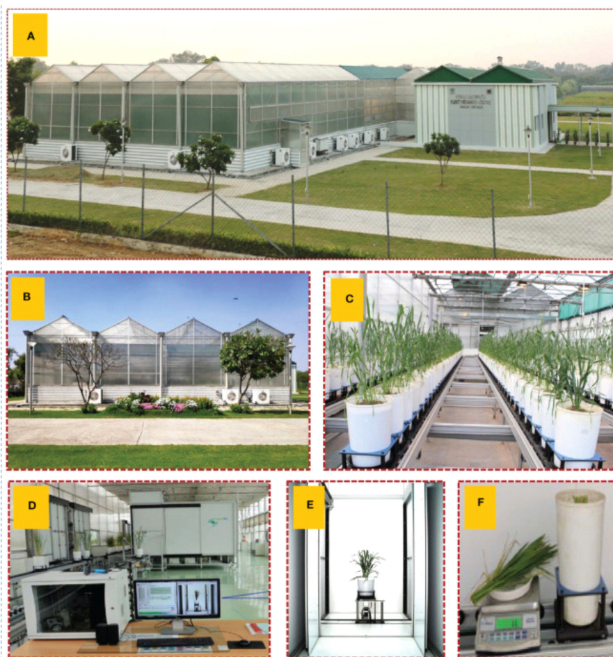
Figure 4. (A) Nanaji Deshmukh Plant Phenomics Center (NDPPC) at ICAR-IARI; facilities like (B) climate controlled greenhouses; (C) experiment for non-invasive biomass prediction; (D) image acquisition and processing; (E) RGB, side view image of wheat plant inside imaging chamber; and (F) Destructive sampling for biomass measurement
