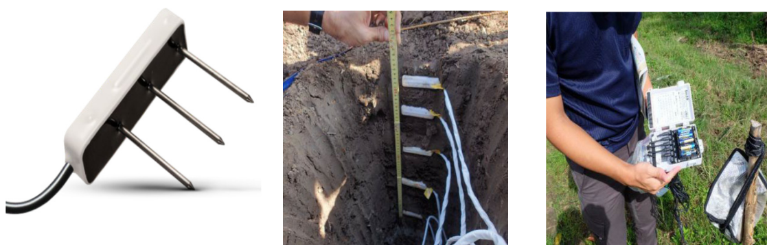
Figure 1. Soil moisture, EC and temperature sensors for continuous measurement of profile soil water and salinity
