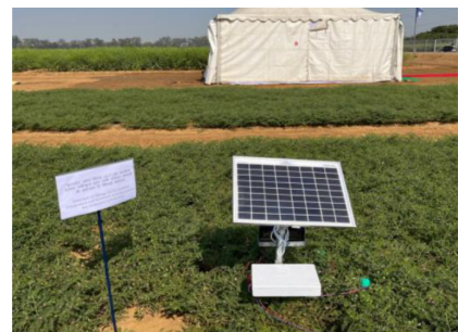
Figure 3. IoT enabled IWMS in chick pea at ICAR-IARI farm, New Delhi
