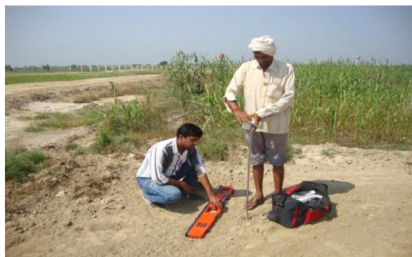
Figure 2b. EM38 measurement in horizontal mode
