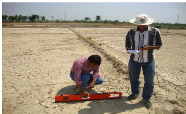
Figure 2a. EM38 measurement in vertical mode
