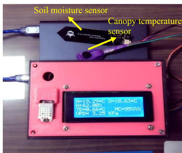
Figure 5. Integrated sensing device with soil moisture and plant canopy temperature sensors
